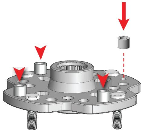
f. Locate a **brake rotor (73-14778)**. Place the rotor on to the hub and line the holes up with the rotor spacers and tapped holes.
