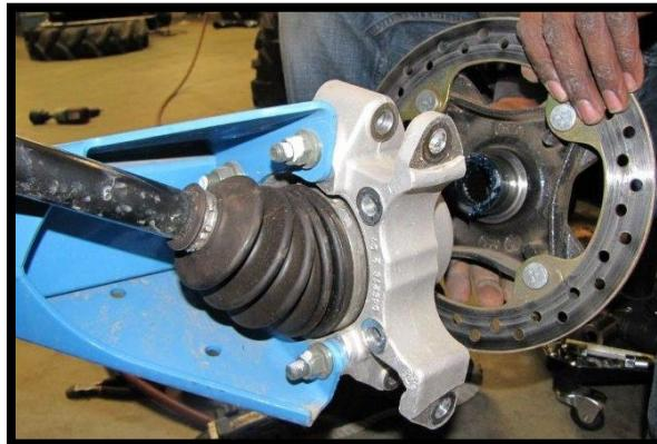
e. Remove the bolts and nuts that attach the rear knuckle to the upper & lower A-arms. (15mm)
