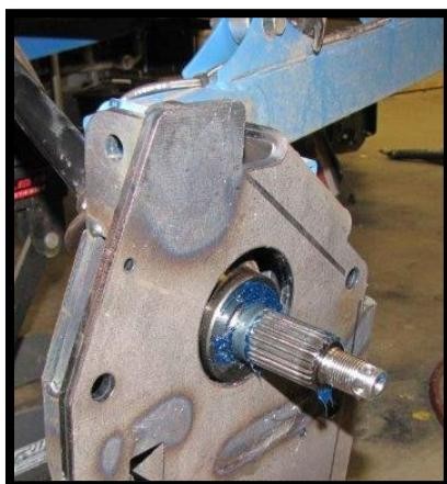
b. Install the backing plate to the trailing arm using **M10-1.25x35 bolts** and **10mm flat washers** on each side. Then fasten bolts with **M10-1.25 lock nuts**. (15mm) [56 ft lbs]
