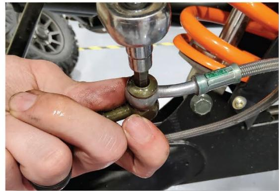
Disconnect the stock brake line from the caliper. Have a container ready to collect brake fluid. Locate the proper BRAKE LINE EXTENSION. Using the supplied button head hex drive banjo bolt, connect the STOCK BRAKE LINE to the BLIND-END BRAKE LINE EXTENSION. Ensure the copper washers are on each side of the banjo fitting.
